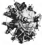
The DeSoto Model 1-477 radial engine above develops 133 hp. The letters on the engine denote: A—water pump; B—all back valve connections; C—auxiliary connections; D—ignition connections; E—all valve connections; F—fuel pump and; G—all fuel connections; H—oil valve; I—fuel tank connection; J—main fuel valve; K—all pressure connections; L—battery connections; M—primary fuel connections; N—bracket connection; O—oil tank.
